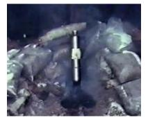
Figure 4: Response to bullet attack - puddle of propellant (liquid)
